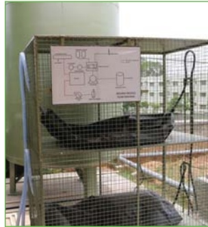
BioUrja's twin balloon biogas compression system
