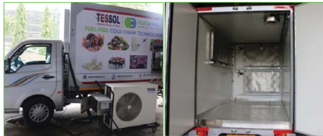
Reefer vehicle using TESSOL's "PLUGnCHILL" solution
